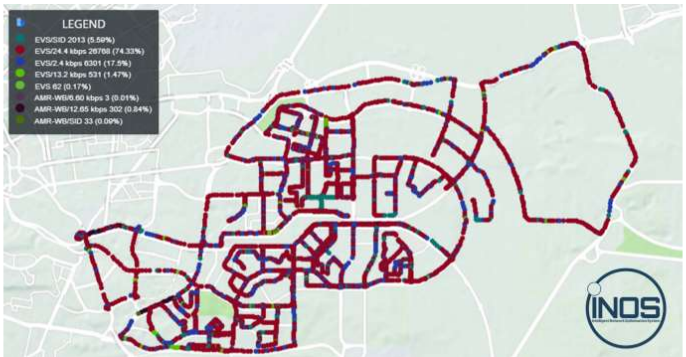
Figure 1 voice codec rate. INOS analysis, for a specific drive test, on one mobile network, in Cairo.
