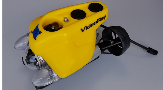
Figure 1. Photo of the VideoRay Pro 4 ROV with attached tether cable. There are three thrusters: One top thruster dedicated for heave, and two rear thrusters dedicated for surge and yaw.
