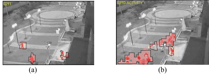
Fig. 5. Temple 1 video (a) showing no activity and (b) showing increased activity due to street fight (ACTIVITY label is shown next to the frame number)
