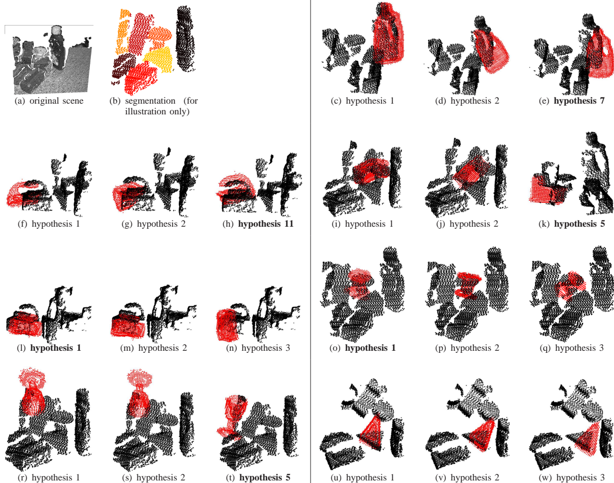
Figure 10. Top sample poses for 7 objects found by the MC-SCOPE algorithm for a cluttered scene. When a “good” pose sample is found within the top 20 samples, the caption under the best sample is shown in bold.
