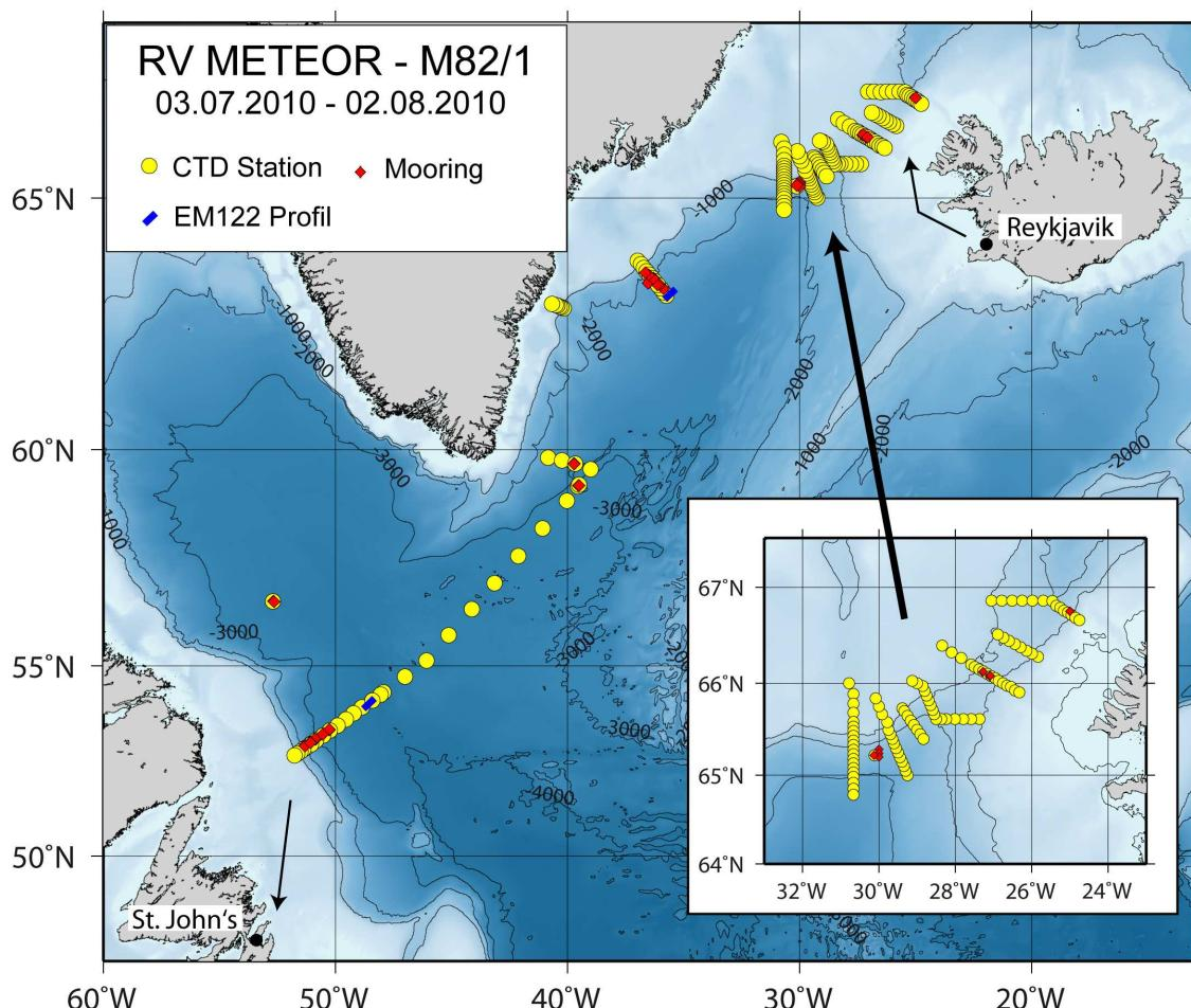
Track of RV Meteor cruise M82-1 in the Labrador Sea, Irminger Sea and Greenland Sound with locations of moorings (red dots), CTD/IADCP casts (yellow dots) and acoustic surveys (blue dots).
