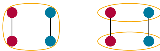
■ Figure 1 Example forest where a cluster of size 4 and two clusters of size 2 incur the same cost. With one cluster of size 4 (left), the inter-cluster cost is 0 and the intra-cluster cost is 4. With two clusters of size 2 (right), both the inter-cluster and intra-cluster cost are 2.
