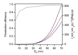
As we can see, particle loss is considerable below 10 nm (up to 40%) but in terms of their contribution to particle volume sampled, these losses are negligible. Most of the particle volume collected was in fact from the highest size bins (upper limit 70 nm). The penetration efficiency curve was added to the supplementary information (Fig. S1).
