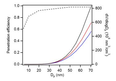
As we can see, a significant number of particles are lost at the smallest sizes (up to 40% below 10 nm) but in terms of their contribution to particle volume sampled, these losses are negligible. Most of the particle volume collected was in fact from the highest size bins (upper limit 70 nm).
