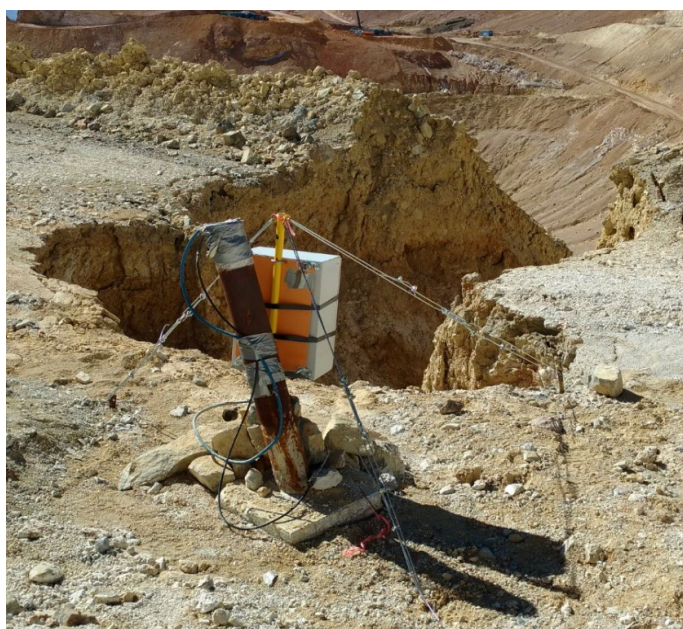
Figure 3: Photograph of borehole 5-1 showing erosional gully that formed during the 2015 calendar year.
