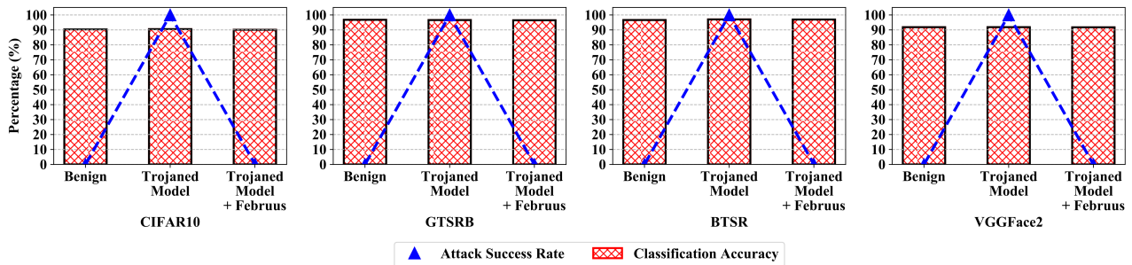
Figure 15: Robustness of Februus on Different Classification Tasks. Februus is highly effective and perform consistently well against backdoor attacks. We can observe attack success rate reductions from 100% to nearly 0% while the classification accuracy is maintained in across the three different classification tasks. Notably, model performance after deploying Februus remains similar to that obtained from benign inputs.
