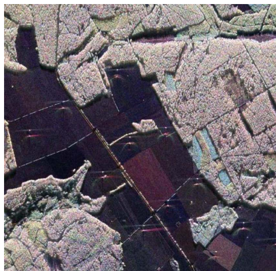
Fig. 15. Rotating windmills close to some forested areas. Image acquired by F-SAR in L-band with 1.5 \times 0.5\text{-m}^2 resolution (blue: VV polarization, red: HH polarization, green: HV polarization).
