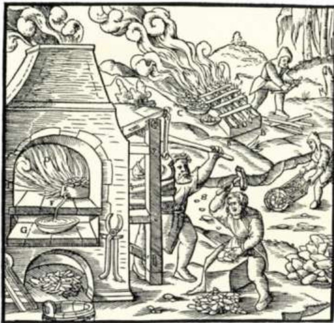
▲ Two illustrations from De re metallica by Georgius Agricola (1494-1555). This was a famous work on mining and metallurgy and these two scenes show the roasting of metal ores.
