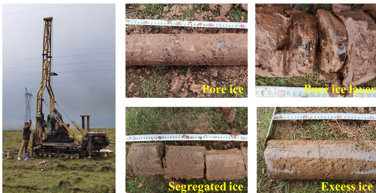
Figure 3. Field permafrost drilling work and various types of ground ice obtained during drilling.
