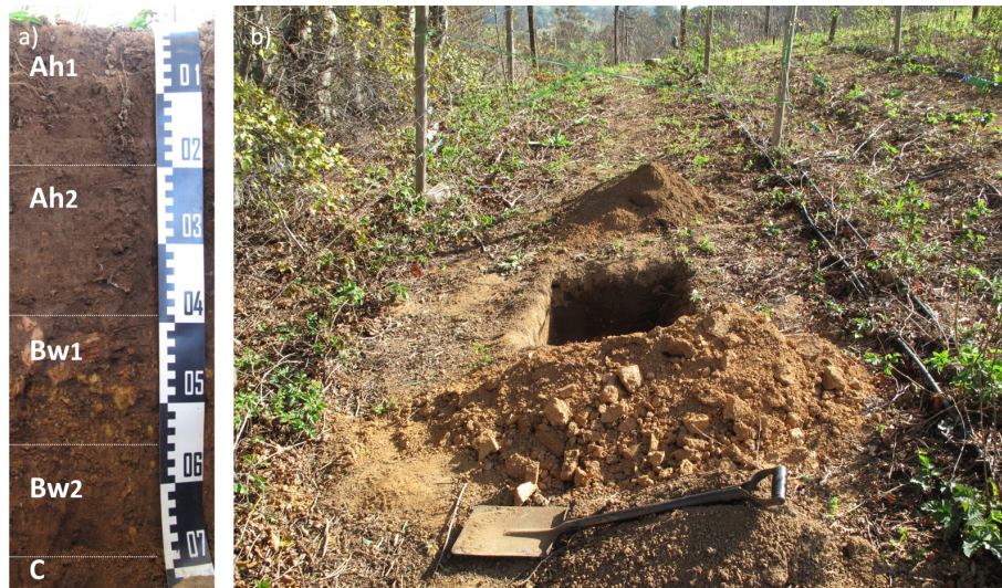
Figure 6. Soil profile: Dystric Cambisol (loamic, colluvic, humic) according to the IUSS Working Group WRB (2015). (a) Profile with the delineated horizons; (b) profile pit between the berry rows.
