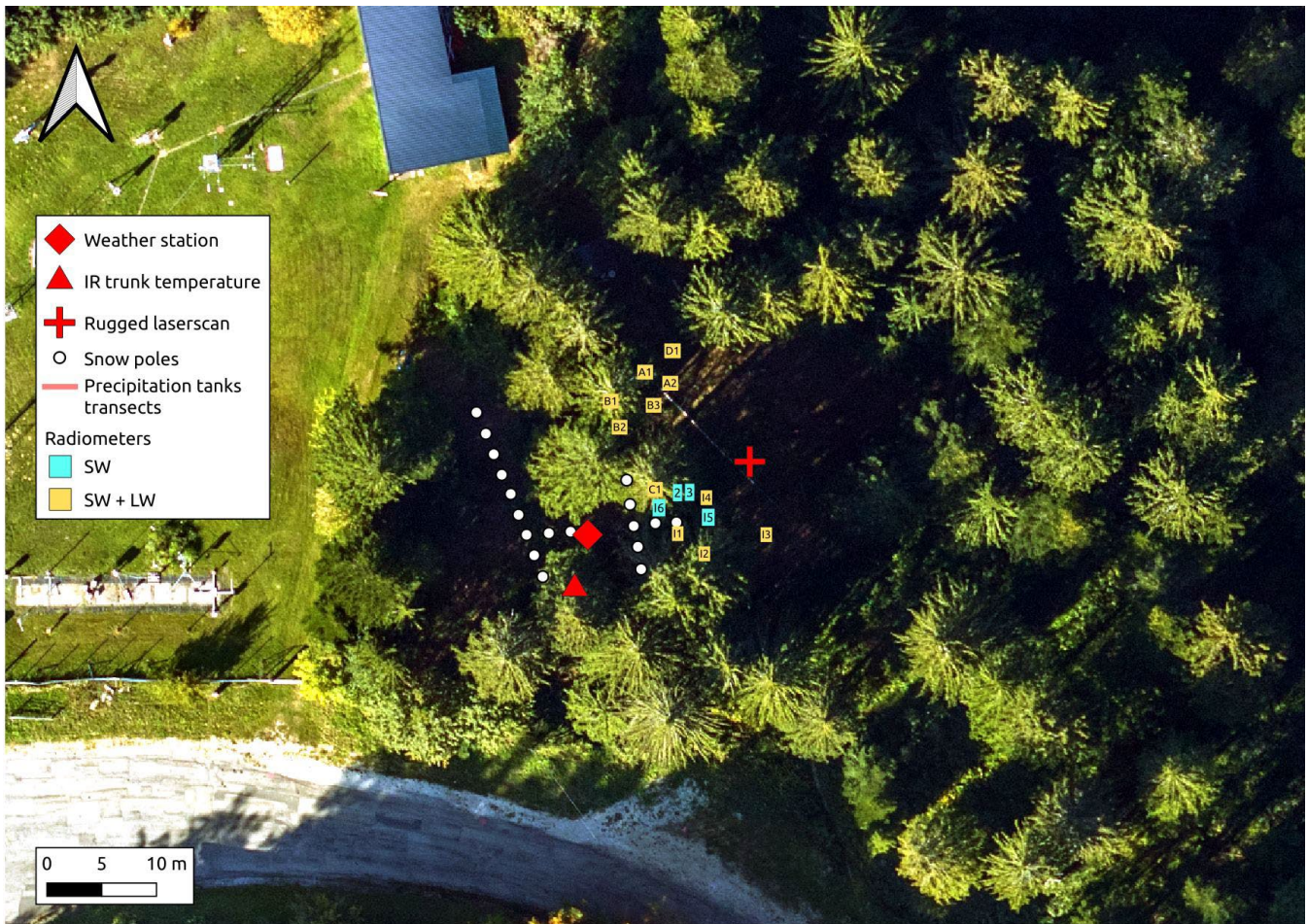
Figure 1: Aerial photographs of the site taken on 30 August 2016, with locations of the sensors during the 2017-18 field campaign. On the left is the meadow with part of the long-term instrumentation for the Col de Porte site. Labels “2” and “3” refer to sensors SW2 and SW3.
