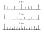
The scale marks must be situated on one side of a real or imaginary line concentric or parallel with the base of the scale and passing through the edges of most of the scale marks.
