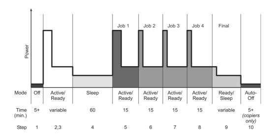
Figure 2 shows a graphic form of the measurement procedure. Note that products with short default-delay times may include periods of Sleep within the four job measurements, or Auto-off within the Sleep measurement in Step 4. Also, print-capable products with just one Sleep mode will not have a Sleep mode in the final period. Step 10 only applies to copiers, digital duplicators, and MFDs without print-capability.
