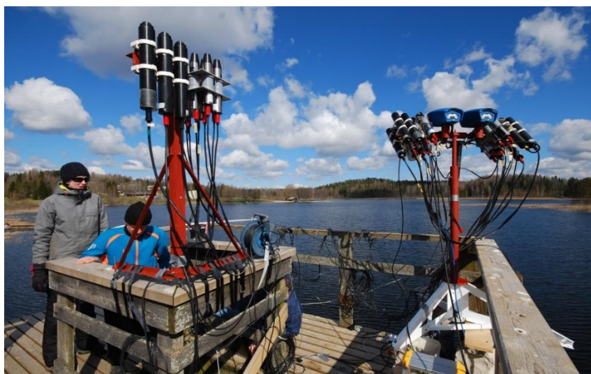
Figure 16. All the radiance and irradiance radiometers were mounted in common frames during the LCE-2 outdoor experiment. Left frame – irradiance sensors; right frame – radiance sensors.
