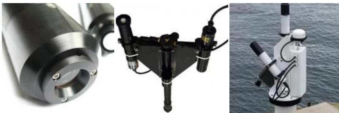
Figure 4-10 Satlantic HyperOCR hyperspectral radiometer (left) radiance and, in background, irradiance sensors (middle) mounted on a free-fall profiling frame (right) mounted on a SAS system with solar tracker for above-water measurements. [source: Sea-Bird Scientific]
