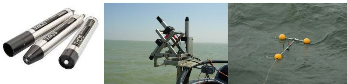
Figure 4-15 TRIOS RAMSES radiometer (left) instruments with fore-optics for radiance, cosine irradiance and scalar irradiance [source: TRIOS], (middle) mounted in 3-sensor frame for above-water radiometry [source: RBINS], (right) mounted in floating system [source: M. Darecki].
