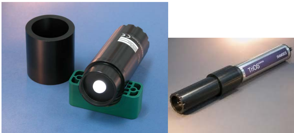
Figure 4-17. White LED-based TRIOS FieldCAL portable calibration source (left) with separate positioning sleeve, (right) fitted on radiance sensor. [source: TRIOS]
