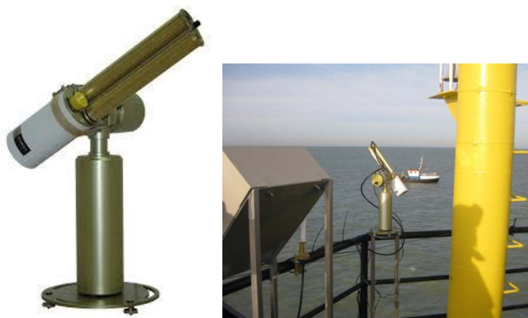
Figure 4-4 CE-318 SEAPRISM system: (left) optical head (white), collimators and pointing robot; (right) RBINS Zeebrugge/MOW1 AERONET-OC site, including to left of image the weatherproof enclosure housing the control box.
