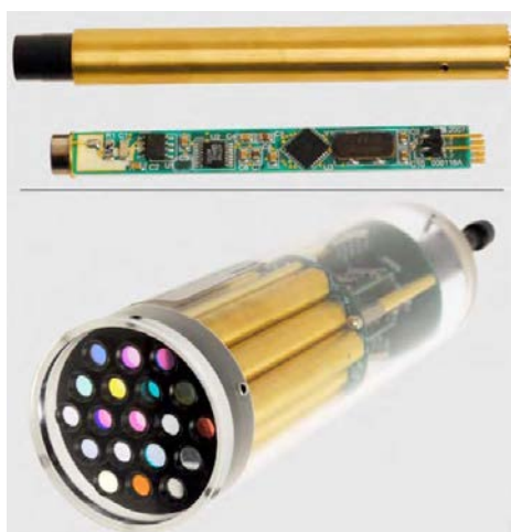
Figure 4-1 (top) An individual microradiometer sleeved in brass. The anodized black section contains a Gershun tube and optical filter stack. (middle) Microradiometer PCA consisting of the photodetector, preamplifier, ADC, microprocessor and RS-485 digital communications circuitry. (bottom) An example C-OPS-style radiance radiometer built using a cluster of 19 microradiometers in a clear acrylic housing. The power supplies and aggregator PCA are located beneath the microradiometer array (photo courtesy Morrow et al. 2010).
