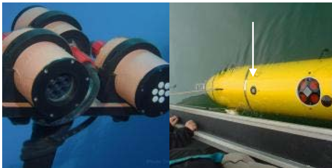
Figure 4-11 Satlantic OCR507 (left) seven channel radiance and irradiance sensors mounted on an underwater frame and (right) seven channel irradiance sensor mounted on a Hydroid Remus AUV. [source: Sea-Bird Scientific]
