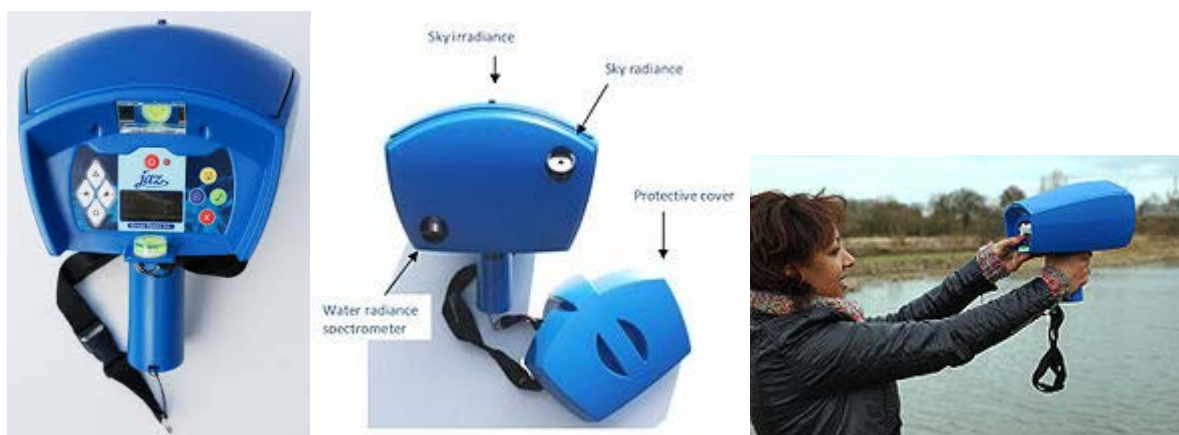
Figure 4-19. WISP-3 radiometer system: (left) back view, as seen by operator, (middle) front view showing radiometer fore-optics, (right) in operation.
