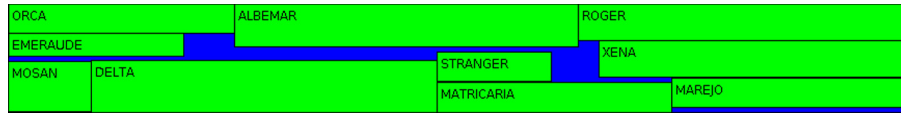
Fig. 8. Example of an instance with 10 ships where less than 10% of the chamber's surface is still free.
