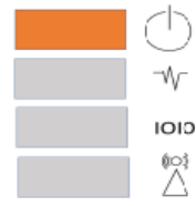
Figure: Power supply does not have redundancy
