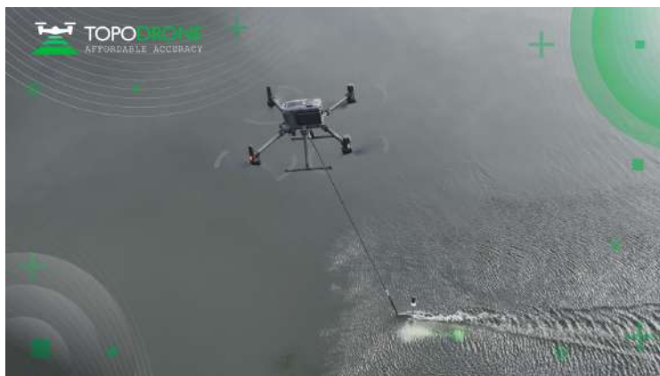
Figure 1: Reservoir surveying with TOPODRONE AQUAMAPPER © TOPODRONE.
