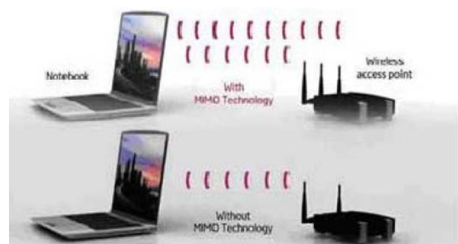
Fig. 1 : MIMO technology uses multiple radios to transfer more data at the same time
