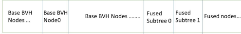
Figure 5: Memory layout of fused BVH. The subtrees from the LOD 1 BVH fused in with the Base BVH.
