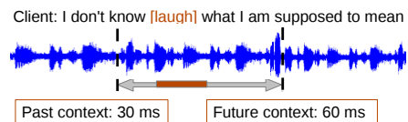
Figure 2: Example of extracting acoustic cues from speech. In this example, we trim the speech starting at 30 milliseconds before laughter begins and 60 milliseconds after laughter ends. This is followed by extraction of prosodic signals and computation statistical functionals on the speech segment.
