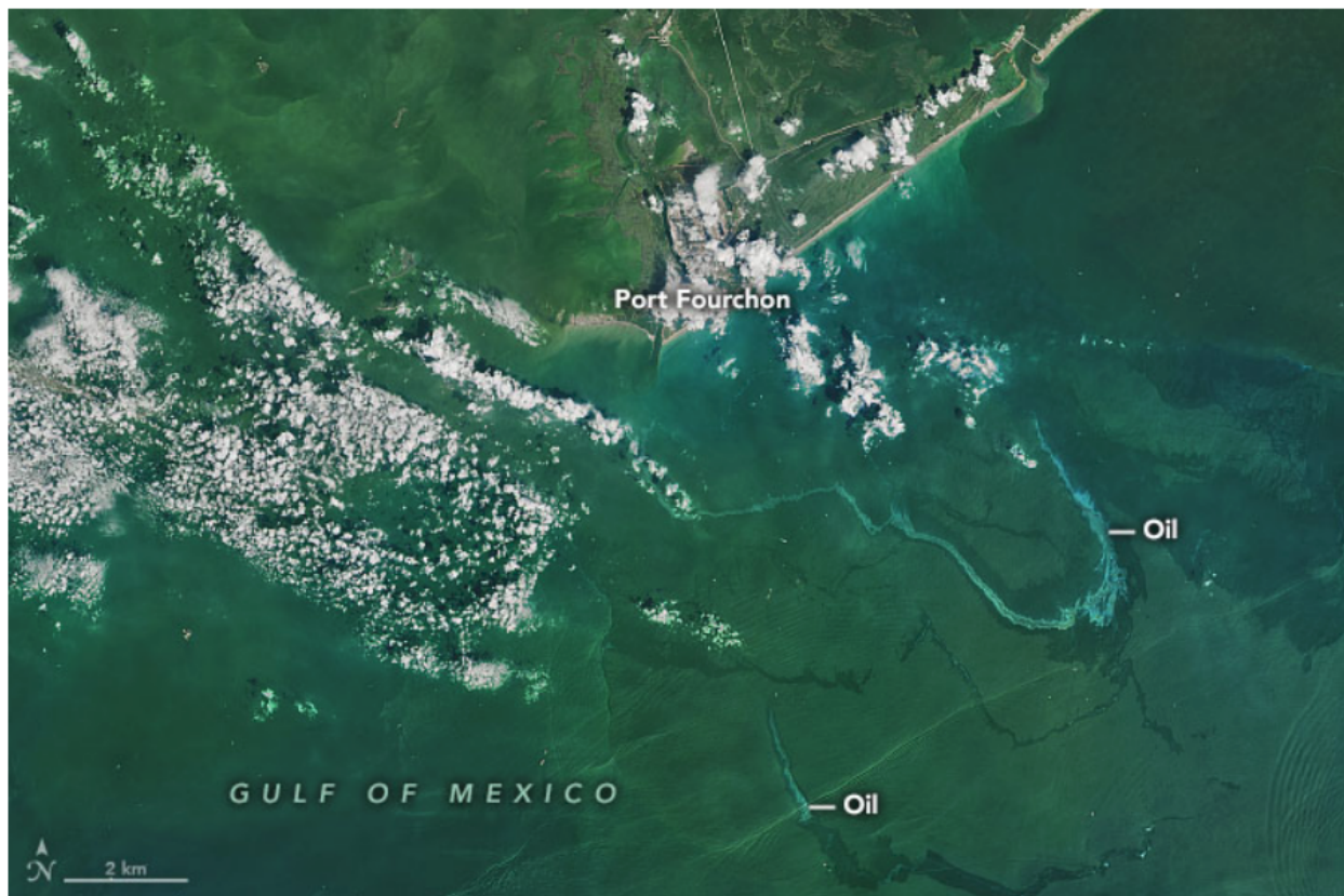
Figure 8. Oil trails visible as blueish lines in this image, as captured from the LANDSAT-8 - OLI satellite and sensor. Photo: NASA Earth Observatory, 03 Sept 2021.
