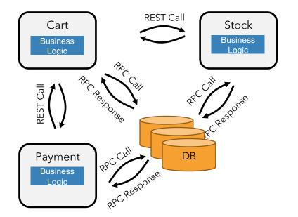
Services are *stateless* Database does the heavy-lifting High latency, costly state access No guaranteed messaging 80% of code in the service layer is error checking. Transactions: Java XA or SAGAs.
