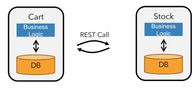
Low-latency access to local state Service calls still expensive Messaging still not guaranteed Not obvious how to scale this out Fault tolerance is hard!
