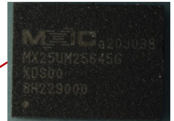
32MB SPI with low-level firmware
