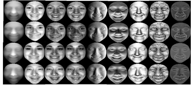
Fig. 2. Illustration of happiness expressions of four 3D face scans with nine kinds of extracted features in BU-EDFE database. And from left to right are the depth maps, 3-channel textured information (R, G, B), 3-direction normal maps (x, y, z), and curvature maps (curvature and mean curvature).
