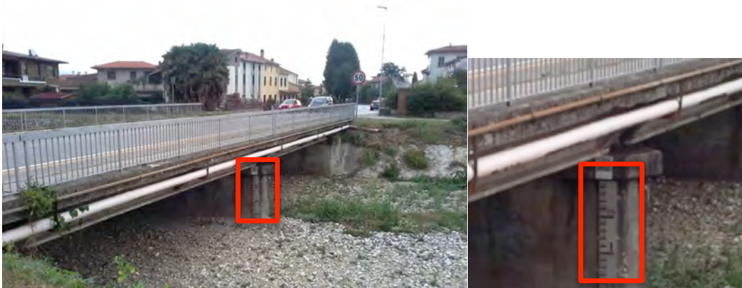
Figure 5. Water level gauge and QR code installed at Marano Vicentino, on river Timonchio (expanded view shown on right).
