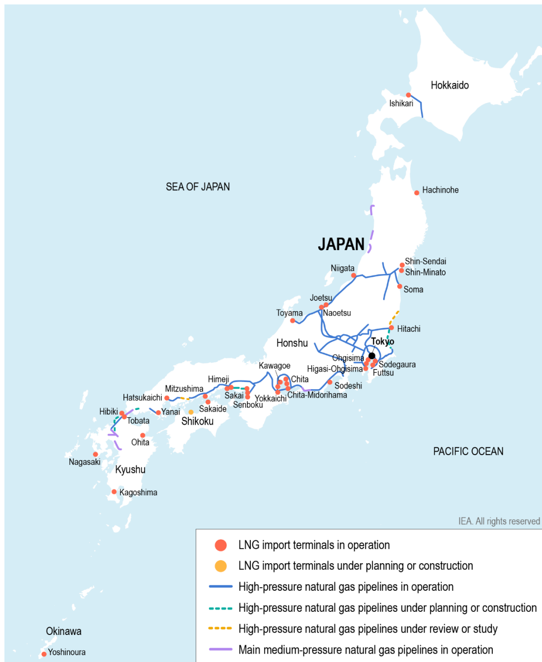
Figure 8.5 Japan's main LNG terminals and pipeline network, April 2019
