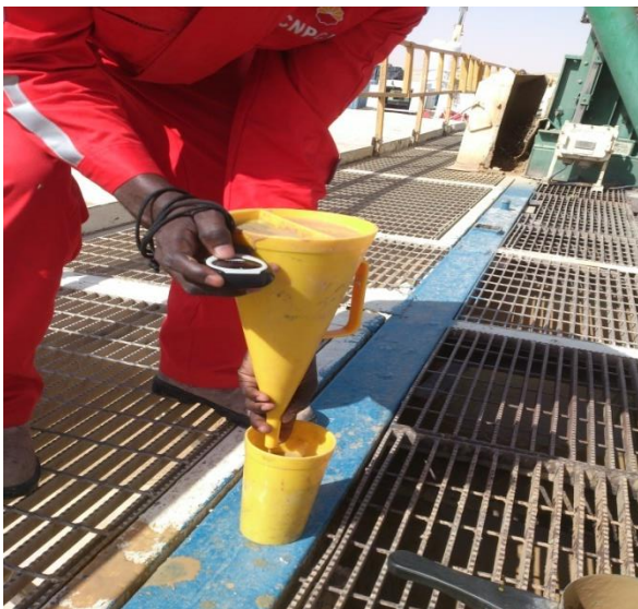
Figure 4. Measurement of mud viscosity using a MARSH Funnel
