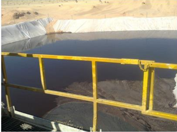
Figure 3. Mud tank used on the Dibella well site
