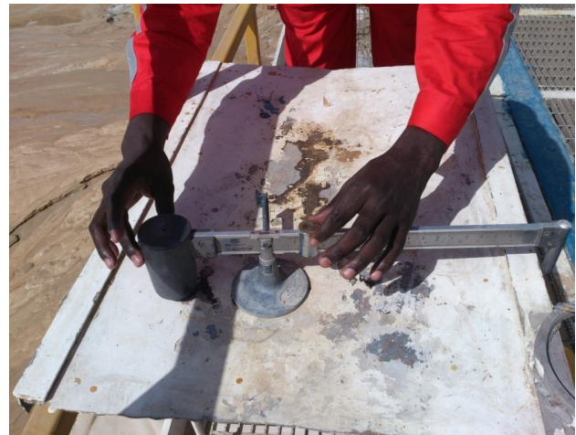
Figure 5: Density measurement of the mud with a densimeter
