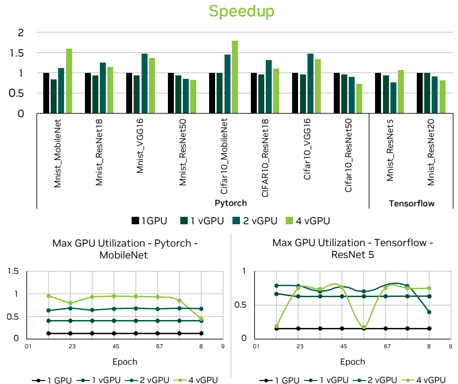
Figure 3. Performance comparisons between physical GPUs and virtual GPUs. Credit: Rong Ge and her students, Deep Learning on vGPUs: A Case for High GPU Utilization and Throughput.
