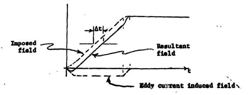
There is a transient condition during the time the magnet current changes from a ramp to flat top whose exact nature can not be determined until the exact magnet program is known. However, from equations (1) and (2)
