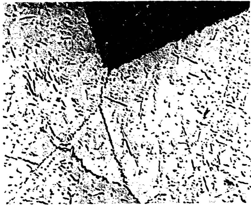
Fig. 15. Tensile Fractures and Microstructures of L-605 Aged for 500 hr and Tested at 540°C. (a) Aged at 760°C, (b) aged at 815°C, and (c) aged at 870°C. Potentiostatically Etched. 1000X. Reduced 5.5%.
