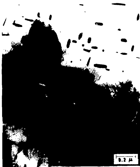
Fig. 2. Transmission Electron micrograph showing \text{Ni}_3\text{Ti} precipitates in an Fe-12Ni-0.25Ti alloy.
