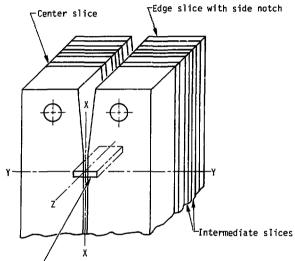
Slice tangent to starter notch root taken to determine  $\sigma_y - \sigma_z$  at the root. Values we e extropolated to the free boundary by thinning several times and recording the fringe values.
