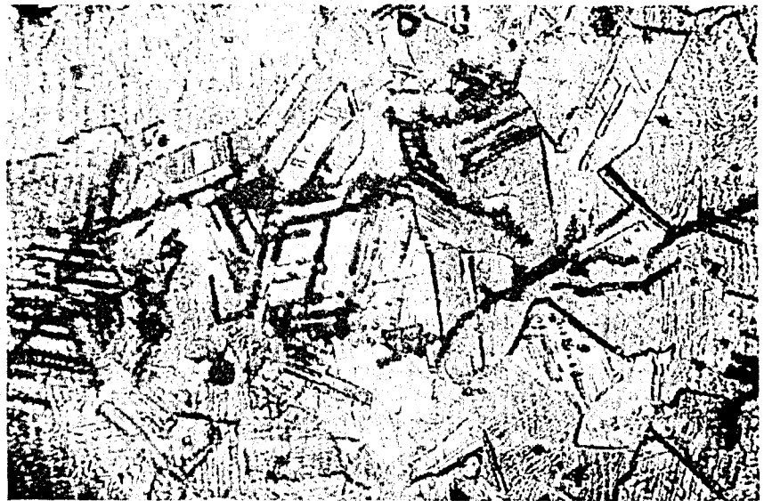
Fig. 16 Microcracks parallel to line markings in irradiated stain- less steel tube. Etched, Mag: 400 X
