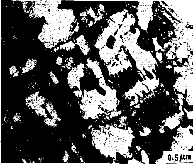
Fig. 2. Reverted \gamma phase after 10 hours at 500°C (TEM). (XBB 762-1740 bottom)
