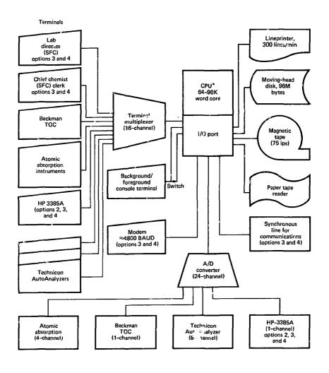
Fig. 1. Schematic of proposed hardware system for Region IV LSB,
