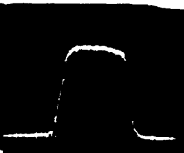
Fig. 5 Output beam with compensation 25 mA/div. 5 μs/div.
