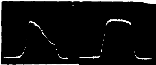
Fig. 4 Output beam without compensation 25 mA/div. 5 μs/div.
