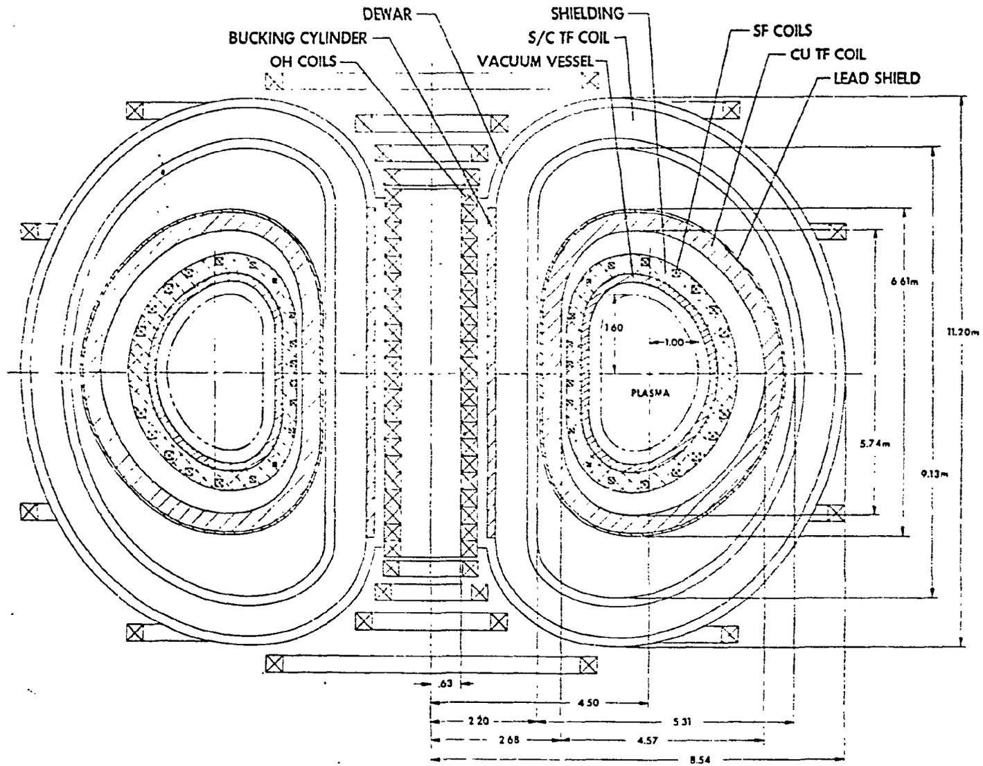
FIGURE 5. REFERENCE TNS WITH COPPER/NBTI TF COILS
