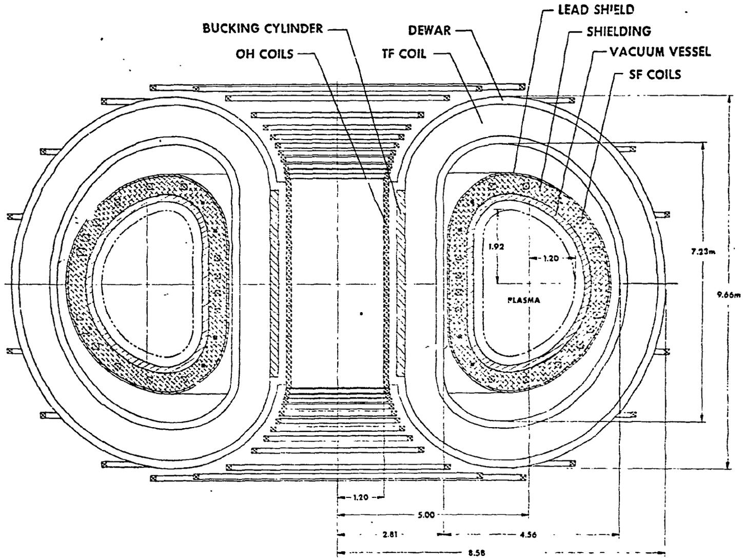
FIGURE 4. REFERENCE TNS WITH  $Nb_3Sn$  TF COILS
