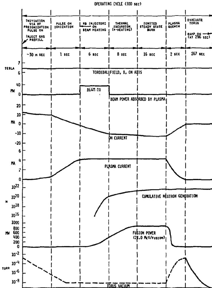
FIGURE 1. THE REFERENCE OPERATING SCENARIO FOR THE TNS OPTION WITH  $Nb_3Sn$  TF COILS IS TYPICAL OF THAT ASSOCIATED WITH OTHER OPTIONS.
