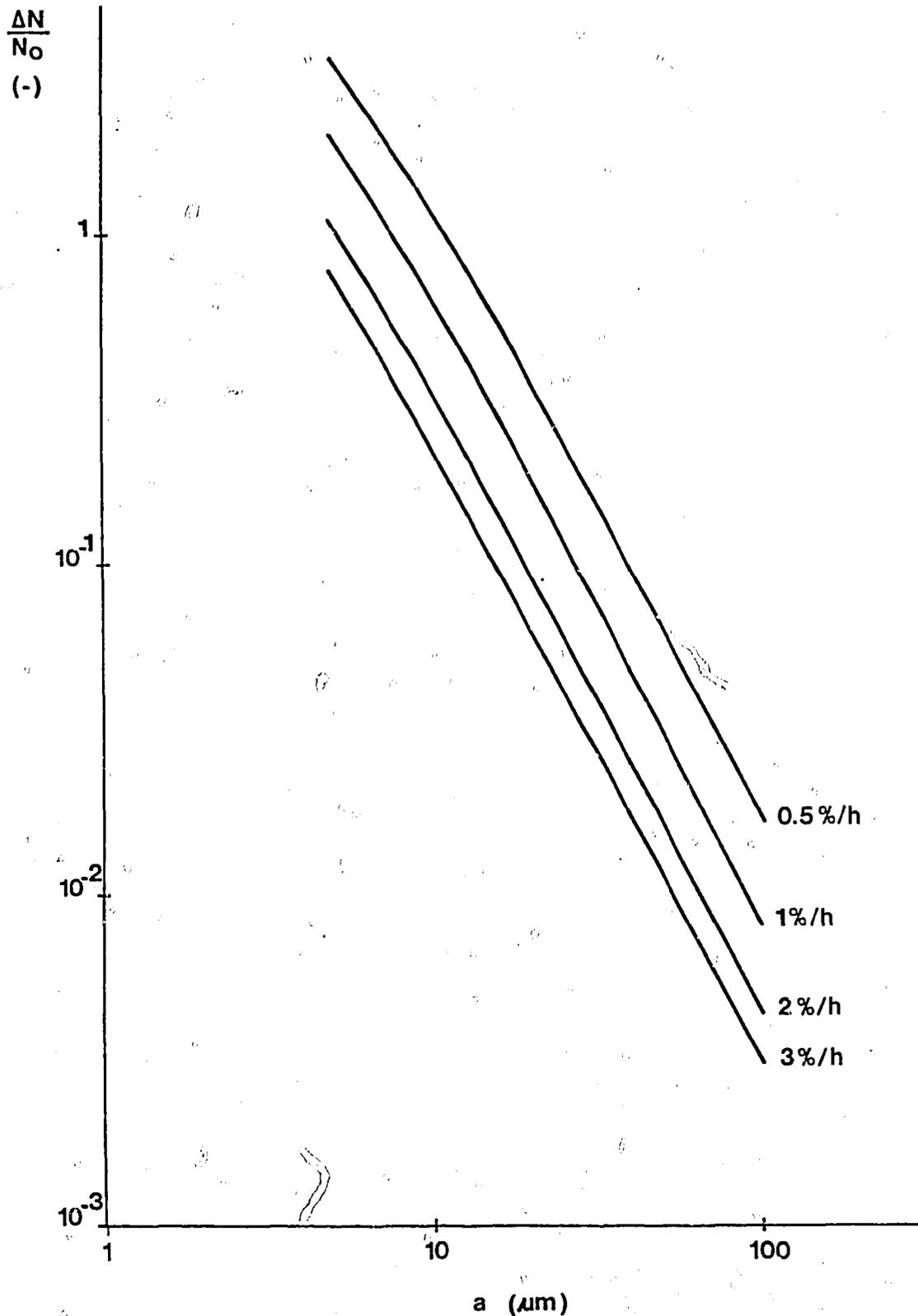
Fission gas release during power ramp as a function of diffusion sphere radius and ramp rate
