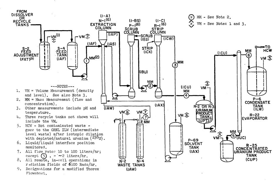
Fig. 1. 233U Solvent extraction system in the Building 3019 Pilot Plant.
