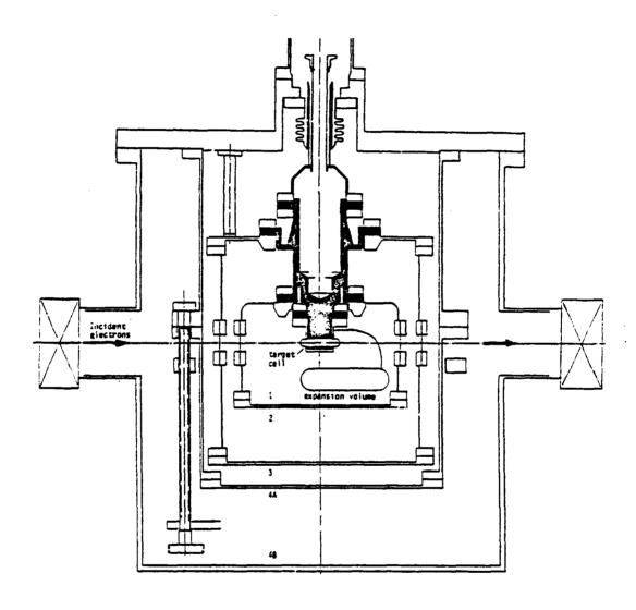
Fig. 2 - The tritium target with its safety envelopes: there are always four concentric envelopes, during transportation and during normal operation. The outer rigid transport vessel can be separated in two parts by remote control, in order to let the beam go through the thin membranes of the inner envelopes.
