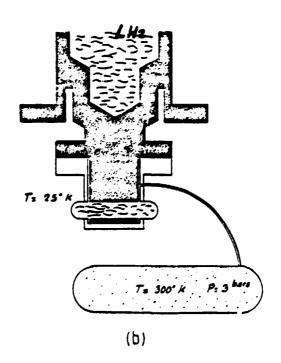
Fig. 1 - The two states of the sealed target : a) out of operation ; b) in operation.
