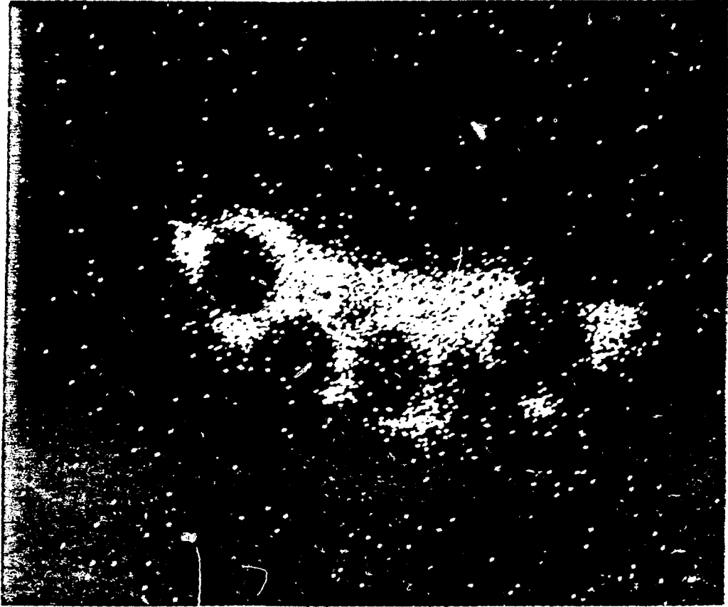
FIG. 6. X-ray Dot Map of Zn from Field in FIG. 4.
