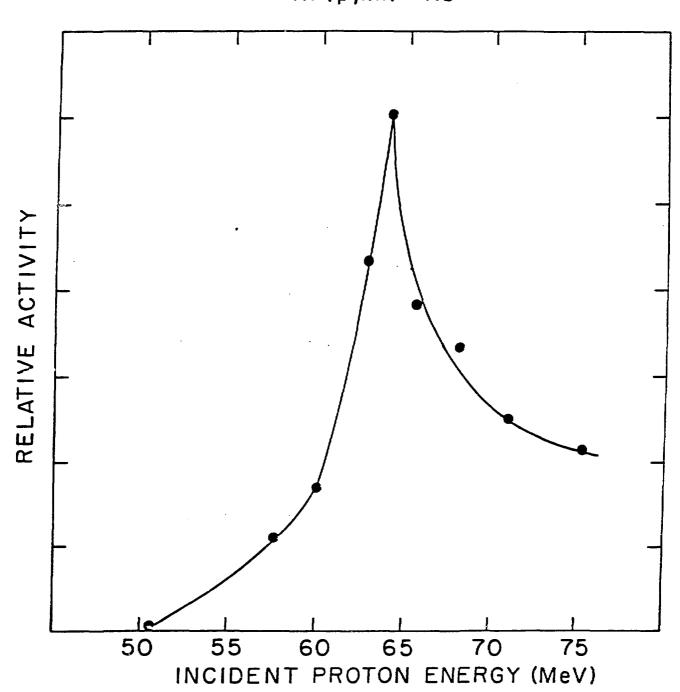
Figure 1. 81 Rb relative production rate vs. energy for a 0.07 g/cm<sup>2</sup> Kr target.
