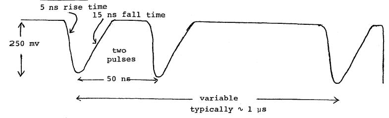
Pulse shape was chosen to simulate that expected from chambers. Repetition rate was typically 1 MHz.
