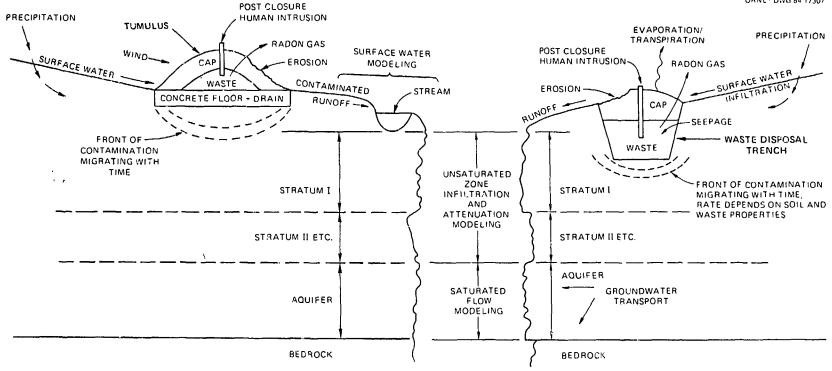
Fig. 1. Schematic of exposure pathways for shallow-land burial and tumulus-type disposal of low-level radioactive waste.
