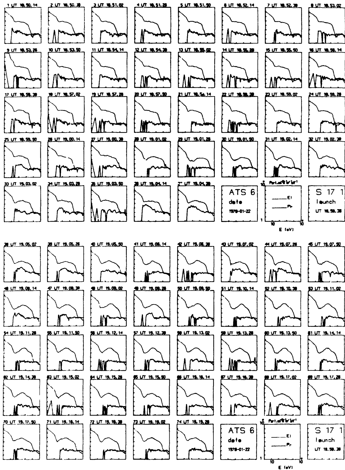
Figure 4.27 Particle spectra obtained from the ATS-6 satellite illustrating the hardening of the flux of electrons during the S17-1 rocket flight (S17-1 launch: 18.58.36 UT).
