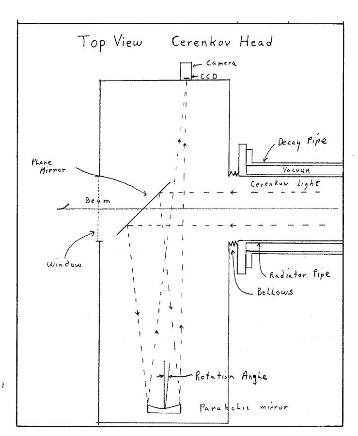
A 45cm diameter radiator pipe is connected to the counter head and penetrates upstream inside the 90cm diameter decay pipe. For safety reasons the radiator pipe must be rigid enough to withstand one atmosphere externally while at a vacuum internally. The pipe is designed in 2m sections with stiffening ribs and baffles at each end. The pipe sections are designed to be assembled and leak tested inside the enclosure as the entire assembly is pushed up into the decay pipe.
